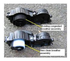
This causes increased crank case pressure which creates an increase in pressure in the sump pushing the oil back up the oil return pipe. This effectively blocks the oil return pipe so the oil entering the turbo through the oil feed pipe cannot escape out the oil drain pipe. As it backs up it is forced out the turbo sideways past the piston rings (seals) into both the turbine housing (exhaust housing) and compressor housing (Air intake housing).
